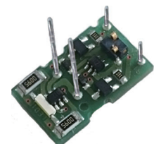
Component mounting from terminal insertion
